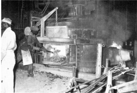
Charging a modest-sized open-arc furnace at Driehoek, Germiston
