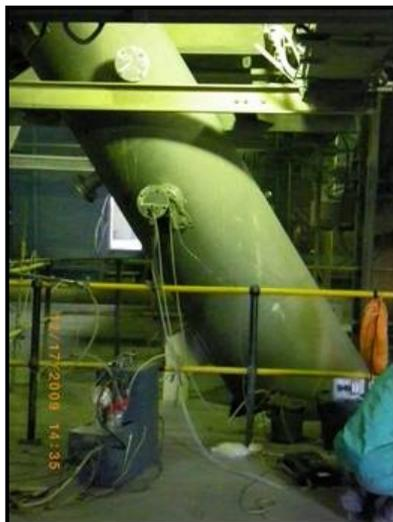
**Figure 1:** Location of gas sampling ports on the slipping floor.
