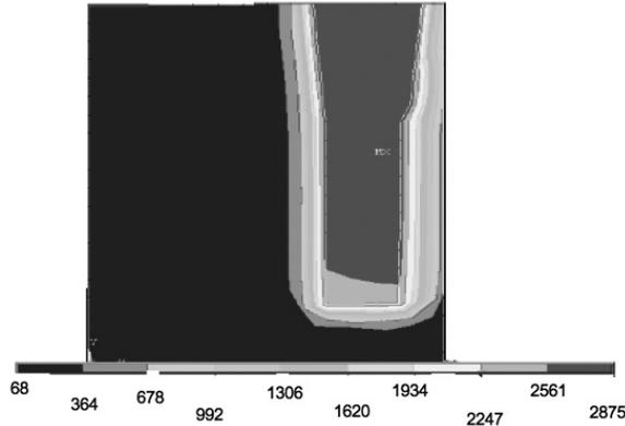
Figure 9: Solidification of the roller at 2 hours
