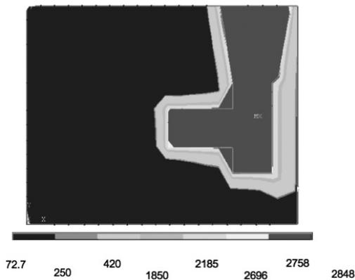
Figure 5: Solidification of the ring at poured temperature (1550°C)
