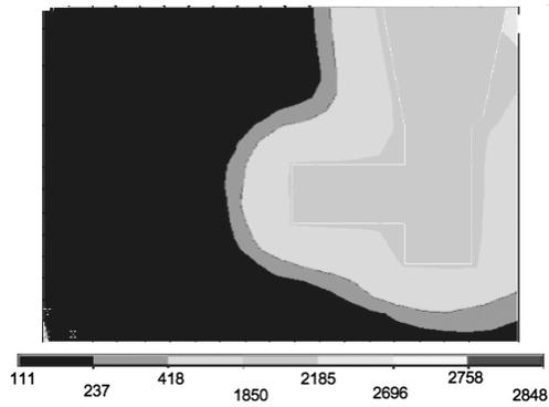
Figure: 7 Solidification of the ring at 6 hours
