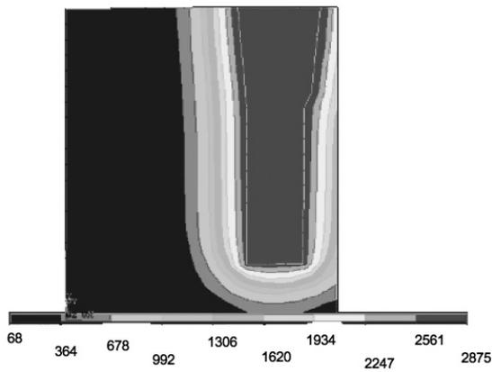
Figure 8: Solidification of the roller at the poured temperature (1550°C) and 0,20 hours
