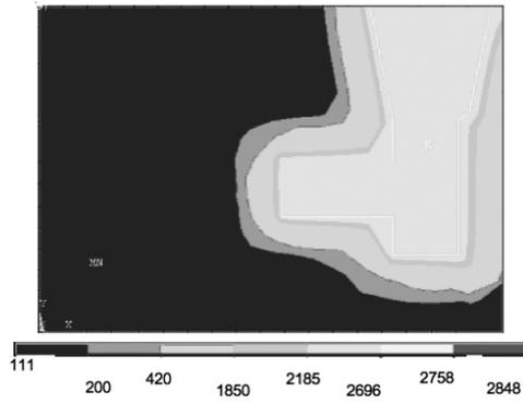
Figure: 6 Solidification of the ring at 2 hours
