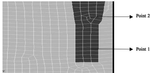
Figure 2: Meshed roller
