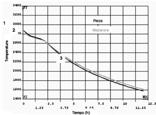
Figure 4: Solidification curves temperature vs. time in the roller
