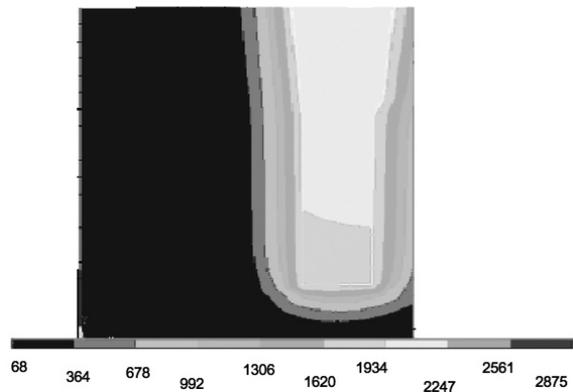
Figure 10: Solidification of the roller at 6 hours
