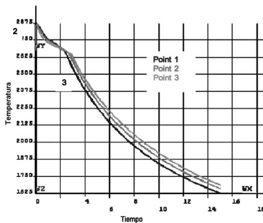
Figure 3: Solidification curves, temperature vs. time in the ring
