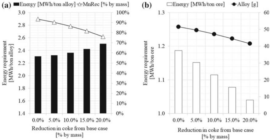
**Fig. 2** Effect of reduction in coke on **a** energy requirement and manganese recovery and **b** energy requirement and alloy produced, where the baseline was 23.06 g coke/100 g ore (Case #7)
