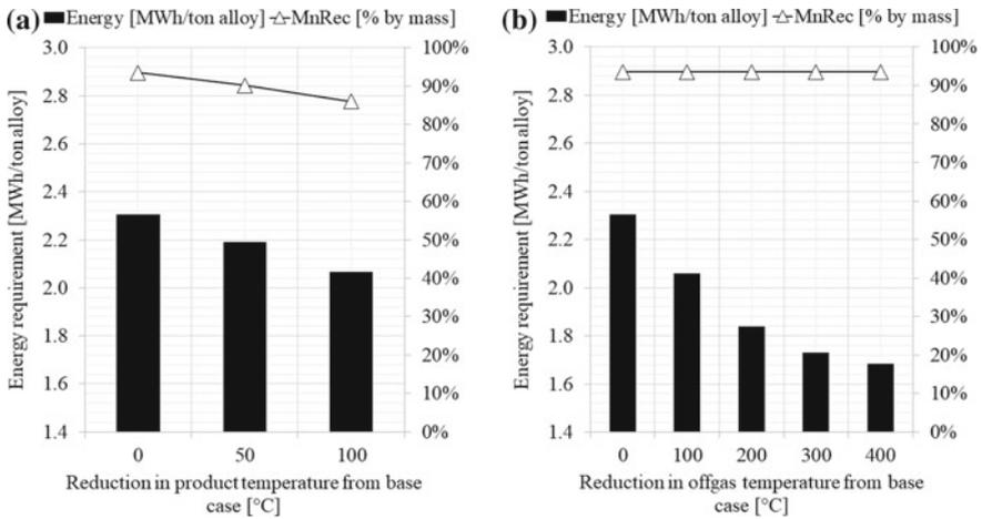
**Fig. 4** Effect of reduction in temperature of **a** slag, alloy, and offgas, and **b** offgas only on energy requirement and manganese recovery where the baseline was 1500 °C for slag, 1400 °C for alloy, and 800 °C for offgas (Case #7)
