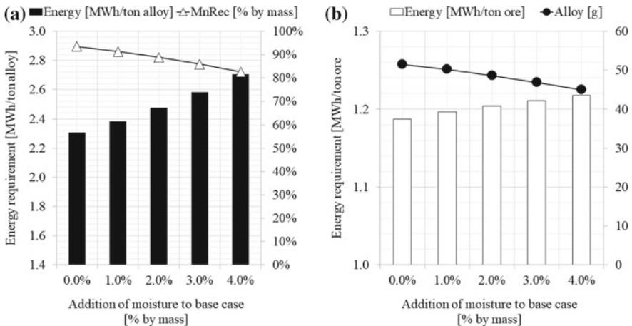
**Fig. 3** Effect of moisture addition on **a** energy requirement and manganese recovery and **b** energy requirement and alloy produced, where the baseline was 0% moisture/100 g ore, i.e., at increments of 1 g moisture/100 g ore (Case #7)
