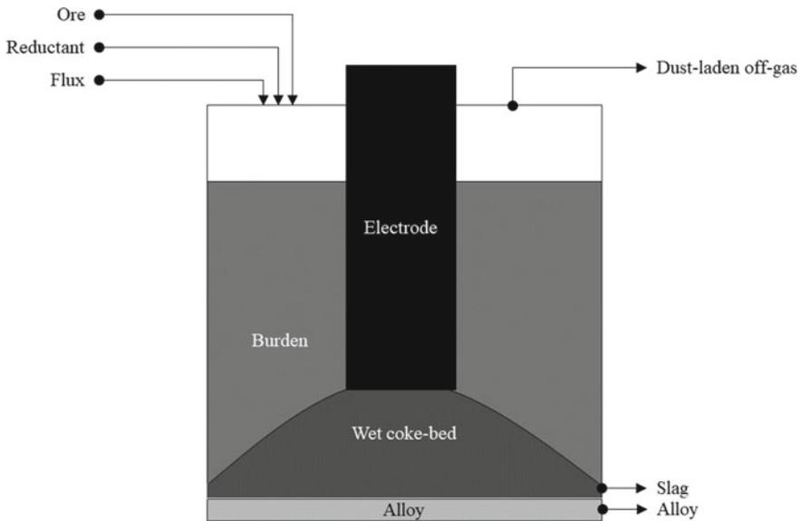
**Fig. 1** Simple schematic of the process flow in a submerged arc furnace utilised in the production of high-carbon ferromanganese
