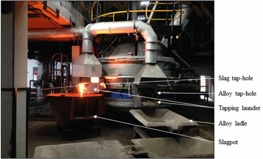
**Fig. 5** Typical ladle arrangement when tapping slag from a slag tap-hole and alloy from an alloy tap-hole in bi-level arrangement
