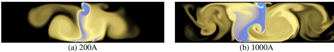
Figure 2: Temperature fields from 2D arc models at 10ms Scale: 2000 K (black) to 15000 K (blue/white)
