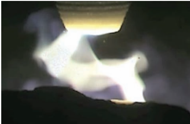
Figure 7—Chaotic arc at 2000 A, 5 cm arc length
