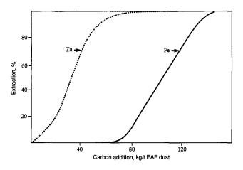
Figure 2—Predicted effect of carbon addition on the extraction of zinc and iron from high-zinc EAF
