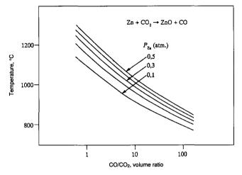
Figure 5—Temperature of the back-reaction of zinc with CO<sub>2</sub> at different CO/CO<sub>2</sub> ratios and zinc partial pressures in the off-gas
