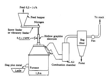
Figure 7— Schematic diagram of the Mintek 1 MW plasma-arc furnace
