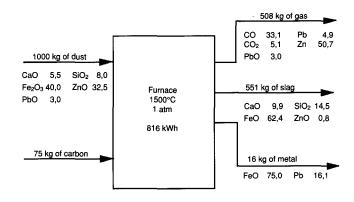
Figure 1—Predicted mass and energy balance for high-zinc EAF dust (all the analyses are given in percentages by mass)
