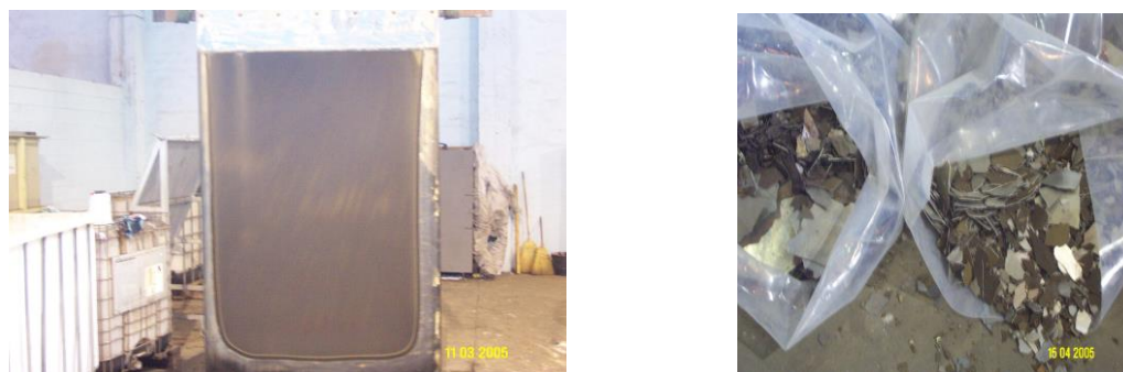
Figure 2: Picture of Mn covered anode (2m x 1.3m, the biggest used till the moment) and manganese flakes
