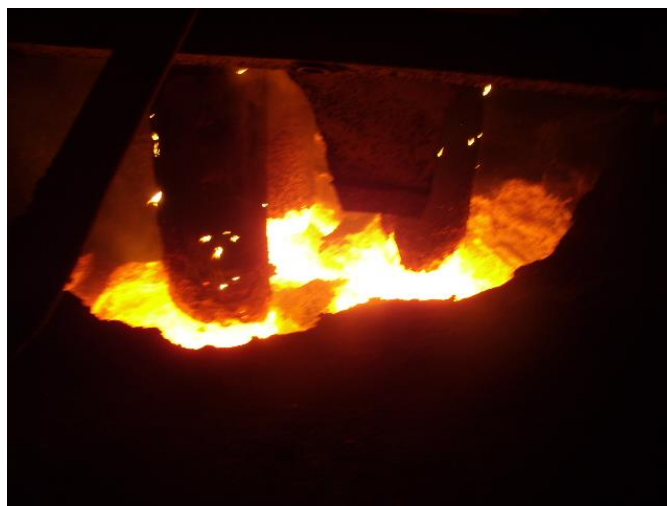
Figure 4: MnC17 screenings melting with an open periodic process
