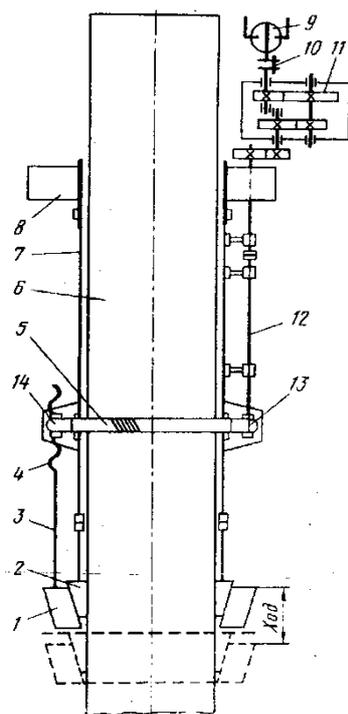
**Fig. 3.** Schematic of clamping contact device operation
