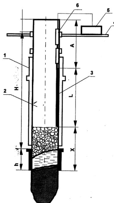
**Fig. 1.** Schematic of thermocouples arrangement in the study of temperature fields of the electrodes 1 - supporting cylinder; 2 - electrode; 3 - a pipe with thermocouple; 4- electrode area; 5 - potentiometer; 6 - protective angles.
