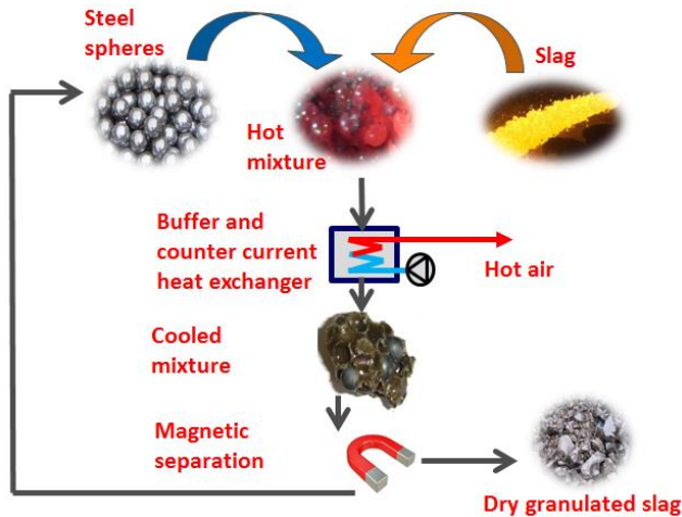
Figure 73: Principle of Paul Wurth dry slag granulation system.
