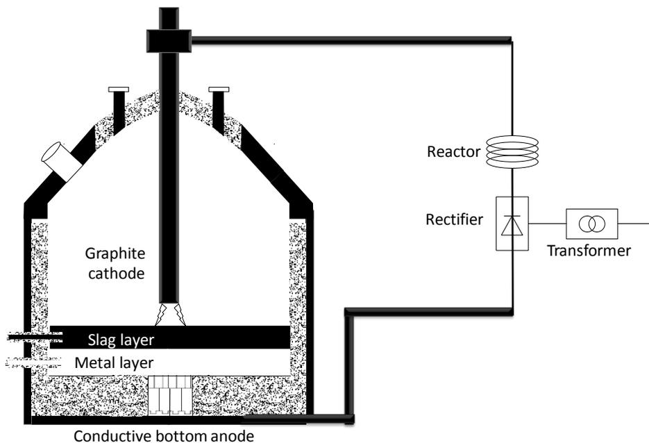
**Figure 58.** Furnace electrical circuit
