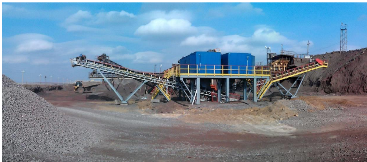
Figure 3: Site for ferromanganese ore sorting based on two MLS sorters. Kazakhstan, JSC “Zhairem GOK”.
