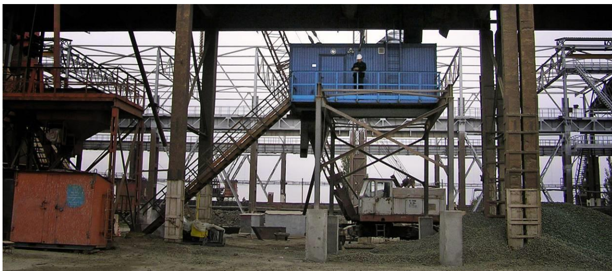
Figure 4: MLS sorter in testing period. MLS is set under the gallery of crushing and screening complex. OJSC “Nikopol Ferroalloy Plant”, Ukraine.
