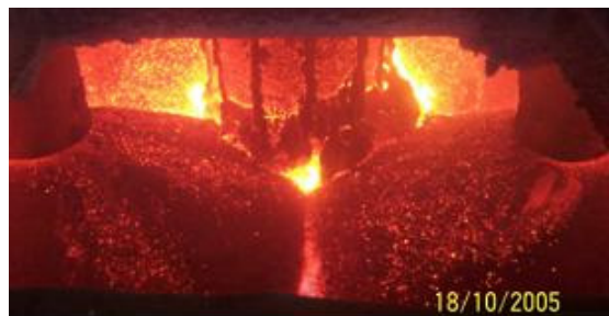
Figure 16: Choke-fed calcine feed piles with combusting reductant-rich valley towards electrode
