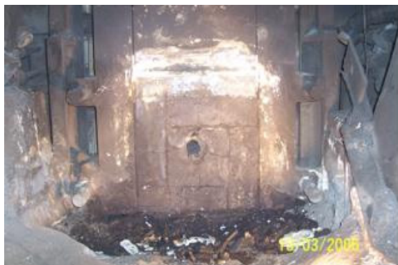
Figure 10: MTB1 – Brick-1 sacrificial replacement after 5 taps. Characteristic “+” shape cracks. Minor crack in surround brick Figure 11: MTB1 – Brick-4 after 219 taps. Multiple drilling of taphole off-centre, coupled with skew lancing
