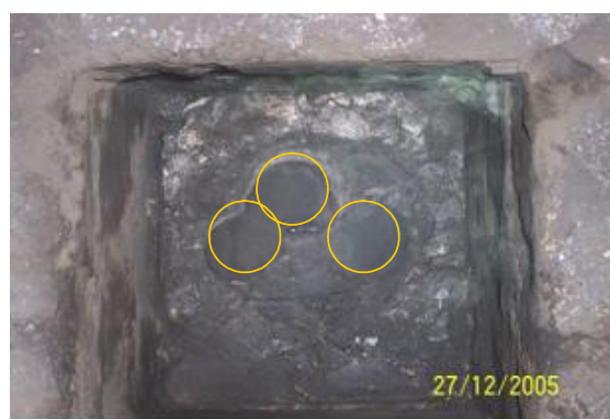
Figure 10: MTB1 – Brick-1 sacrificial replacement after 5 taps. Characteristic “+” shape cracks. Minor crack in surround brick Figure 11: MTB1 – Brick-4 after 219 taps. Multiple drilling of taphole off-centre, coupled with skew lancing
