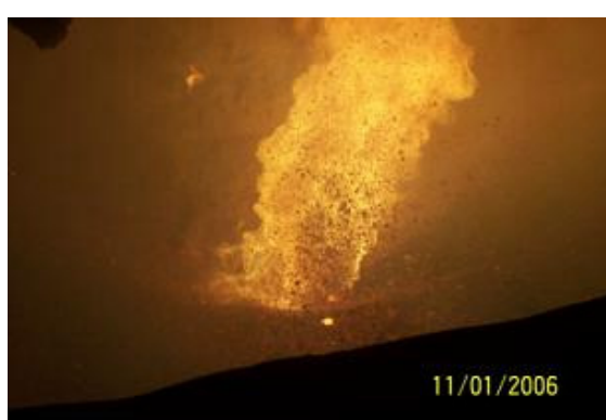
Figure 18: Generation of product gas sufficient to cause ejection of calcine feed
