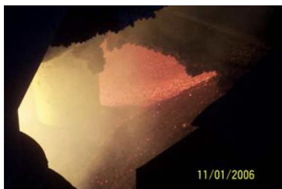
Figure 19: Arc flaring resulting from a combination of higher impedance operation and loss of calcine “shield” around the electrode
