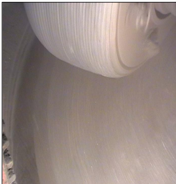
Figure 7: The Loesche mill rollers
