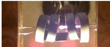
Figure 2. Industrial mould flux sample completely melted at 1400 °C on the thermocouple tip in the additional heating coil.
