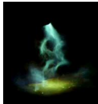
Fig.6 'Pretzel-shaped' arc in air on a graphite block
