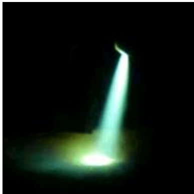
Fig.2 4 kA arc in air, struck on a graphite block
