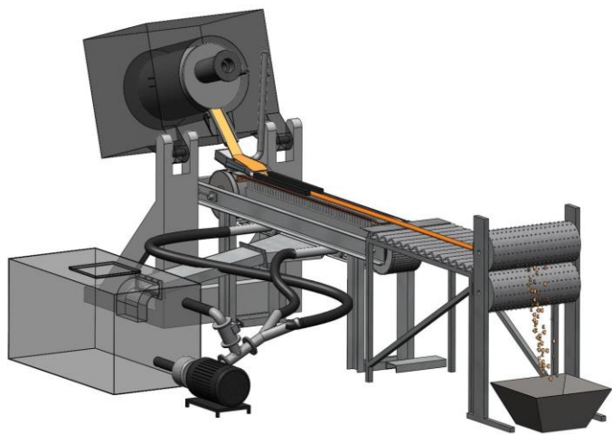
Figure 4: Strip caster at Elkem Technology, principal sketch. Figure courtesy of Elkem Technology.
