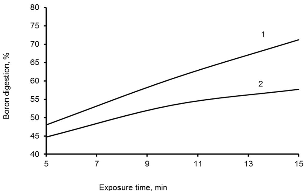
**Figure 2:** Relationship between the boron digestion and exposure time of melt at 1650°C and 2% calculated content of boron in alloy: 1 - calcined Colemanite in powder form; 2 - pelleted calcined Colemanite.
