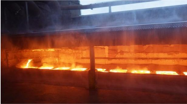
**Figure 8:** Permanently mounted water sprays along the casting bed roof. No fume is escaping from under the roof.
