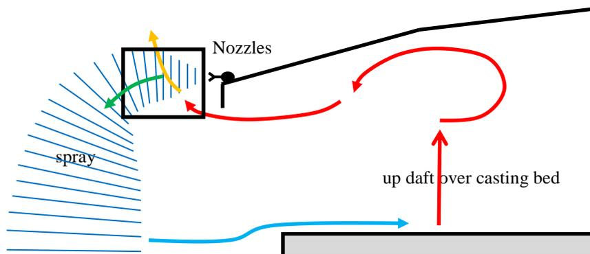
**Figure 9:** Expected flow across the casting bed
