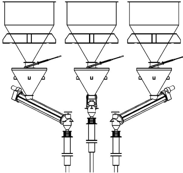
**Figure 2:** 60 MW Furnace Raw Materials Feed System
