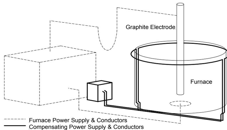
**Figure 5:** Arc Compensation System
