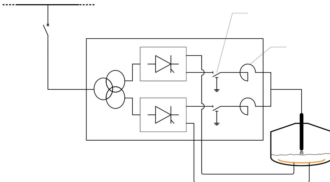
**Figure 4:** Single line diagram of furnace power supply
