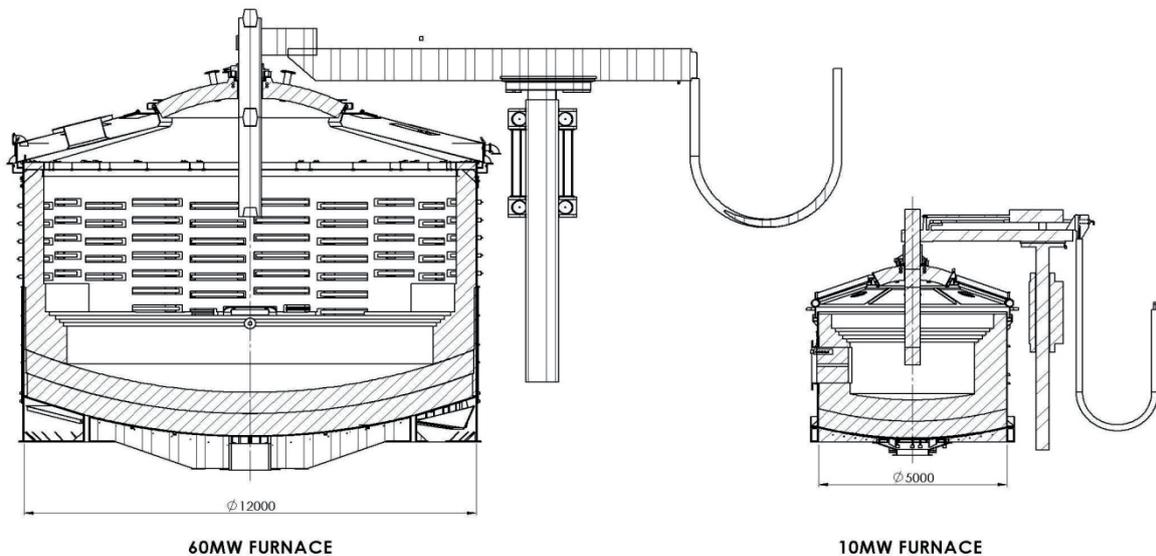
**Figure 3:** 60 MW DC Furnace & 10 MW DC Furnace
