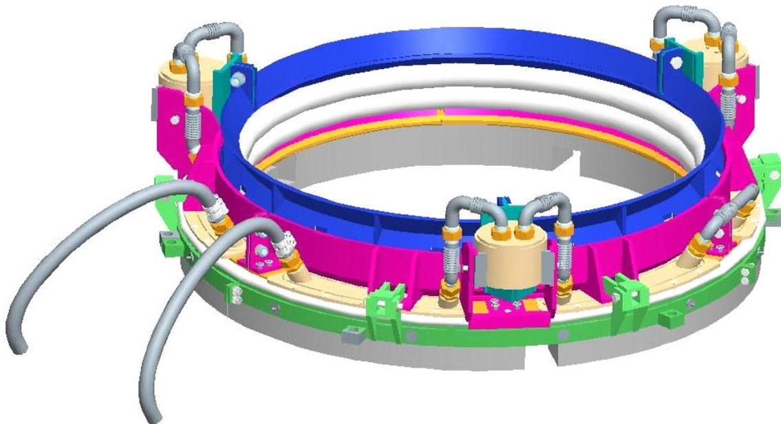
Figure 5: Electrode Smoke Seal
