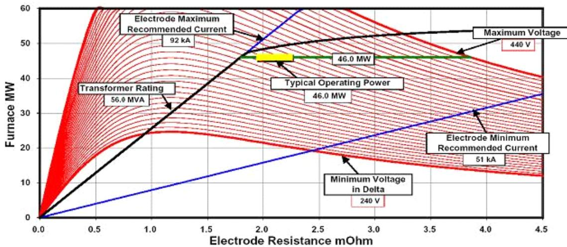
Figure 1: Furnace Operating Graph
